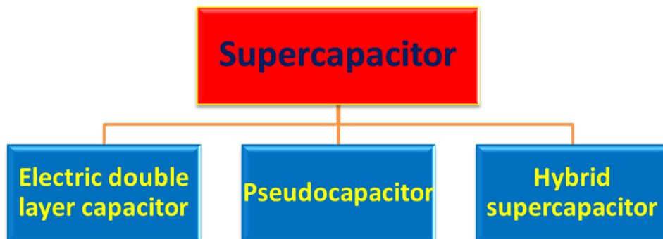
Figure2.3 Schematic of Classification of Supercapacitor
