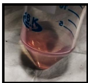
Figure 2.2.2: Pink colour developed in TCC and sodium sulphate containing soil filtrate after dark incubation due to dehydrogenase activity
